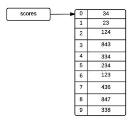
The pseudocode above will create an array with 10 **elements** (spaces). Each element will then be initialised with the values given. A diagram of how this is stored in memory is shown above on the right. To alter one element, for example the first element, we can use the following code:  $scores[0] \leftarrow 23$
